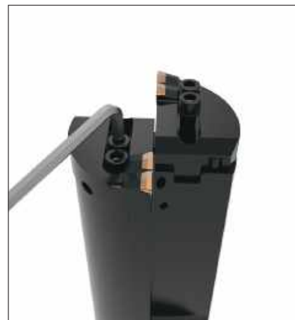
Step 3: Tighten the mounting screws on the cartridge to 11-14 ft-lbf (15-19 N-m).
